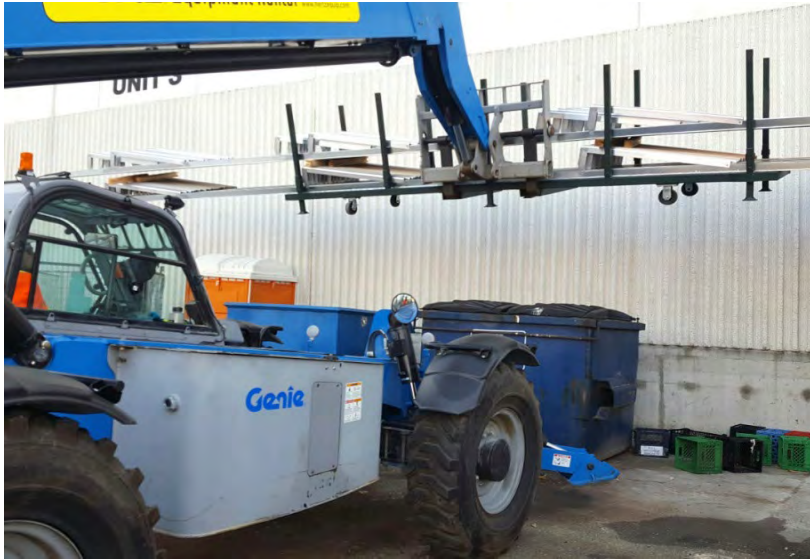
Telescopic Handler hoisting a holding rack with assembled base rails.
