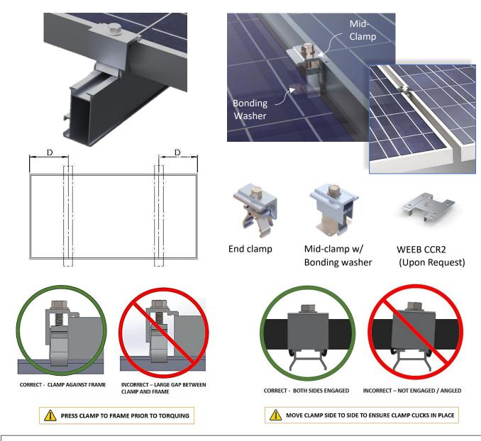
See construction package for details on clamp zones. TerraGen makes every attempt to ensure that the module clamping zones of the module manufacturer are met. However, ultimately it is the responsibility of the customer to verify that the module warranty will be maintained.
