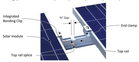
Due to undulations on the roof surface, the angle between the thermal break and the rails may be too large (>2 deg) to allow sliding of the rails on the splice. If this occurs, then the splices on either side of the rail which are not thermal breaks should be Tek screwed to lock them in place.
