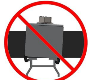
INCORRECT – NOT ENGAGED / ANGLED
