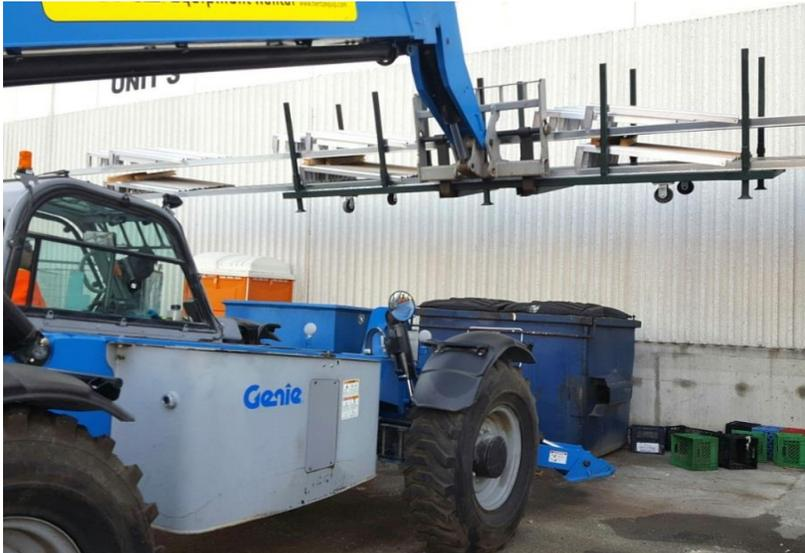
*Telescopic Handler hoisting a holding rack with assembled base rails.*
