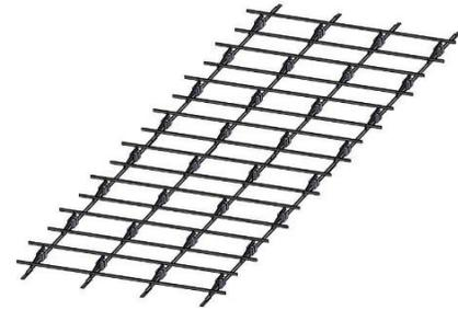
The maximum overhang amount is also specified in the construction package and it is measured from the edge of the mounted panel to the base rail. A minimum of 2" of top rail is required past the end of the module on the starting side.
